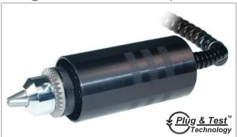
Series R50 smart sensors measure bi-directional torque for a wide variety of applications across virtually all industries. Contain a Jacobs chuck for up to 0.5 in [12.7 mm] diameter samples, bits, or fixtures. The sensors can be used as hand held devices, or mounted to a test stand. Capacities available from 10 ozFin to 100 lbFin [7 to 1150 Ncm]. Compatible with Mark-10 model 5i and 3i indicators (sold separately) through unique Plug & Test<sup>™</sup> technology.
