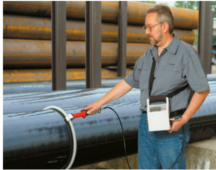
Porosity detection on pipelines
