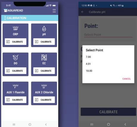
Within the calibration section all fitted sensors calibration options will be displayed, including sensors fitted to the AUX sockets.
