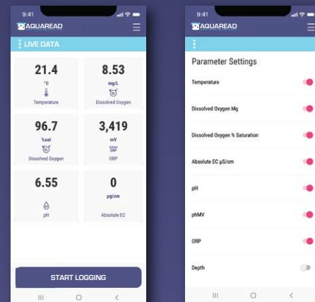
Displayed on the Live Data screen are all of the currently measured readings coming from your connected Aquaprobe.
