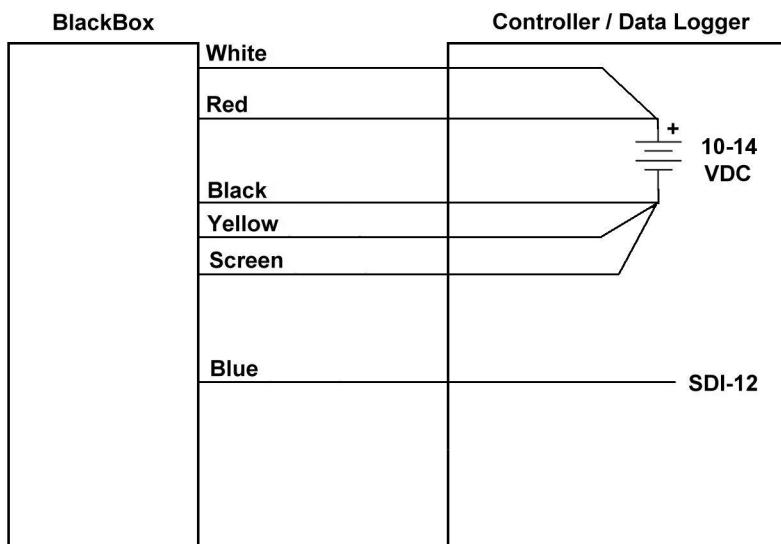
All cores not shown must be cut back and isolated
