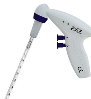
Figure 4, handheld motorised pipette unit with serological pipette attached
