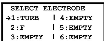
The Fluoride (F) electrode should have been assigned to an AUX socket when it was fitted. Move the pointer to F then press the OK or right arrow key to select.
