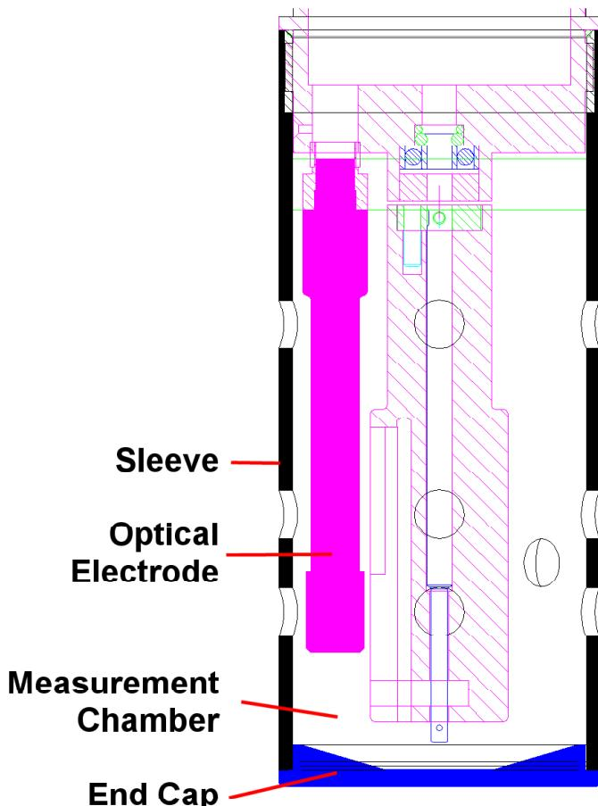
A perfect example of this is calibrating with the end cap removed then measuring with the end cap fitted (or vice-versa). By changing the physical characteristics of the measurement chamber, you also change the calibration and response of the electrode.
