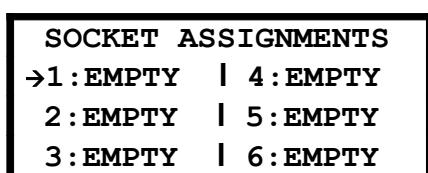
Using the up and down arrow keys, select the AUX socket you wish to assign then move the cursor to the right by pressing the right arrow key. When the cursor has moved to the
