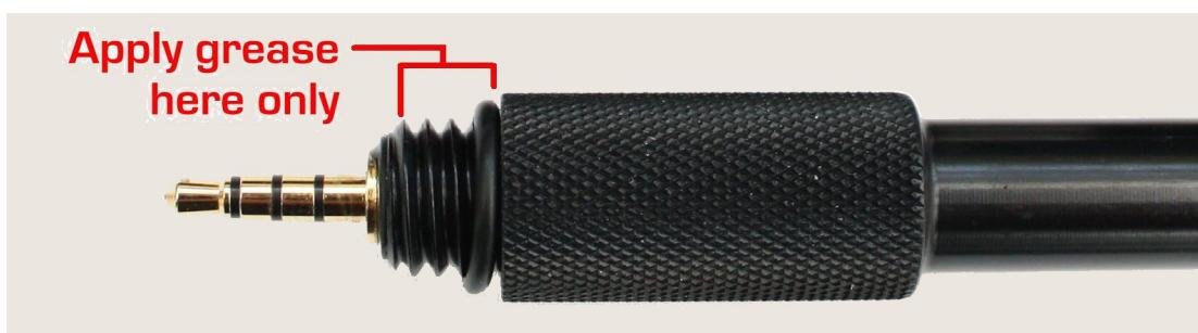
**ENSURE NO GREASE IS APPLIED TO THE GOLD CONTACTS.** Using a clean cloth or tissue paper, polish the gold contacts ensuring they are completely clean. Carefully insert the electrode into the AUX socket and tighten firmly until the O-ring is completely compressed.
