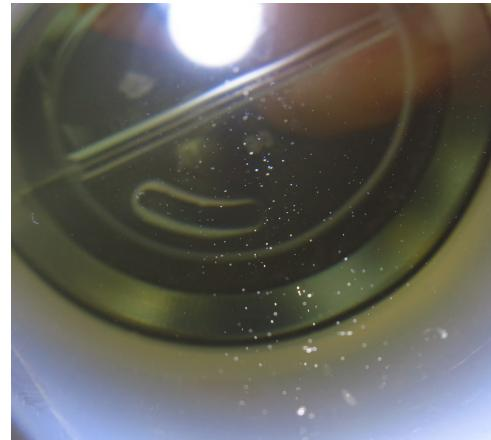
If your zero calibration water is aerated, allow it to stand for a while until the air has all dispersed, then re-insert the Probe and re-calibrate.
