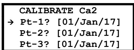
Calibration point 1 (Pt-1) is the warm 10ppm point. Calibration point 2 (Pt-2) is the warm 100ppm point. Calibration point 3 (Pt-3) is the cool 10ppm point.
