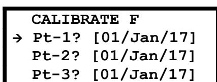
Calibration point 1 (Pt-1) is the warm 0.5ppm point. Calibration point 2 (Pt-2) is the warm
