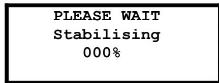
The Meter will wait until the readings are stable, then it will send the calibration command to the Probe, where the calibration takes place. During calibration, the Calibrating screen is displayed and the progress counter counts up. If the calibration is successful, the counter will reach 100% and the following screen will be displayed.
