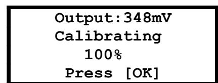
The Calibration Report on the top line displays the voltage output from the ISE electrode in millivolts (mV). This value is stored in the Probe's memory and can be recalled at any time. See section [10.7. Calibration Data Storage and Retrieval](#). Press OK then ESC repeatedly to return to normal reading mode.
