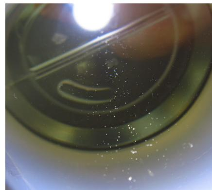
The photograph to the right was taken in a calibration bottle after fresh water was poured in. The bubbles are clearly visible in the light beam. This level of aeration will register the equivalent of around 5NTU as each bubble is seen as a solid particle.
