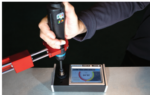
A run down adapter is required when testing power tools with the EZ-TorQ III.
