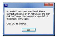
This message appears after opening the software if no instrument is detected. Confirm that the instrument is connected, powered on, and configured appropriately.
