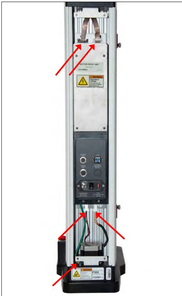
Locations of connectors, ground wire, and bracket
