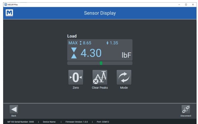
▲ View real-time, peak, and average load data, and zero (tare) and clear peaks.
