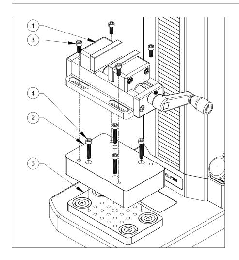
The G1106 vise grip is designed to secure test samples for various compression and tension measurement applications. It may be mounted to Mark-10 test stands with a 25-hole base plate, such as pictured at left.
