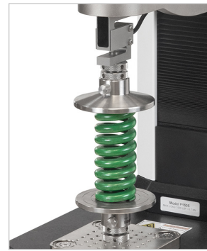
Compression spring testing
