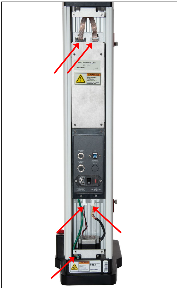
Locations of connectors, ground wire, and bracket
