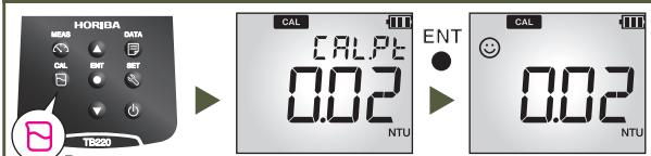
4. Repeat steps 2 and 3 for each standard solution vial. After completing the four calibration points, the screen will switch to measurement mode.
