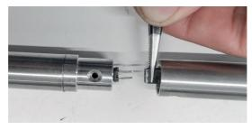
Now insert the connector of the extension into the socket of the basic unit. (The socket can be held with tweezers, for example.) Make sure that the connector is pushed all the way into the socket.
