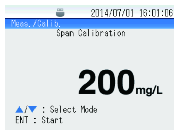
Fig. 23 Start of the span calibration mode
