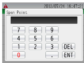
Fig. 73 Span Point screen
