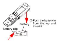
1 Slip the end of the battery into the Battery clip.
