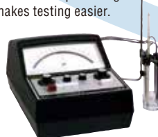
M-5 (benchtop) conversion from vacuum tube to semiconductor allows miniaturization and development of fast response meter
