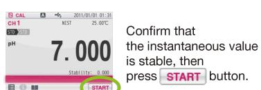
When the **Hold** indication changes from the blinking state to the lit state, calibration is complete.
