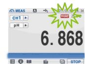
When the **Hold** indication changes from the blinking state to the lit state, measurement is complete.
