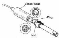
3. Tighten the nut firmly until the nut is totally tight on the sensor head.
