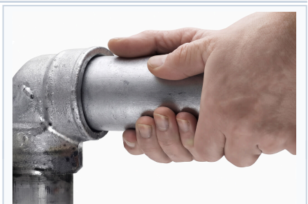
3. Fitter inserts pipe into fitting. Gap-A-Let® ring automatically assures the minimum gap (1/16") to meet requirements of ANSI 31.1 Section III, ASME and military codes
