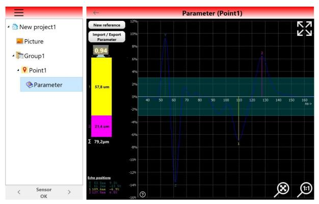
The signal contains a number of positive and negative impulses, including the coupling echo impulses and the echo impulses of the searched echoes at the layer boundaries.
