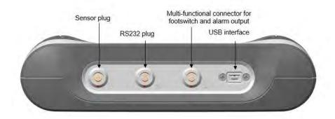
The multifunction socket is used to connect the foot switch or alarm transmitter. The USB socket is used to connect a USB cable to transfer readings or - in connection with the power supply unit - for mains operation and for charging the internal battery.
