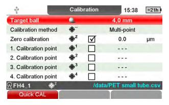
MiniTest FH uses AI to detect the diameter of the measuring ball inserted in the zero cap and automatically performs a zero calibration for this ball diameter.
