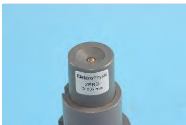
Zero calibration standard with inserted target ball
