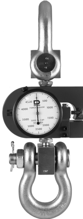
Figure 2.3 Tensile model with adapters and shackles
