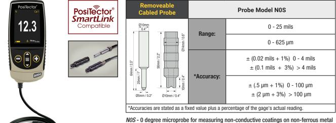
*NOS* - 0 degree microprobe for measuring non-conductive coatings on non-ferrous metal substrates (aluminum, copper, etc.). With our smallest measuring tip and best thin-film accuracy, this instrument is ideal for measuring on small parts, hard-to-reach areas, or close to edges.
