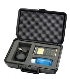
Complete Kit: The TI-25LTX is supplied as a complete kit with the gauge, probe, 4 oz. bottle of coupling fluid, 2 AA batteries, NIST-Traceable Calibration Certificate, and operating instruction manual — all in a foam-fitted carrying case.
