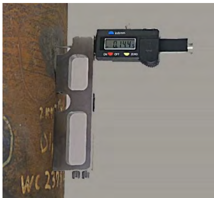
Magnetic V-Groove Base will hold the Gauge in any position: Vertical, Flat or Overhead
