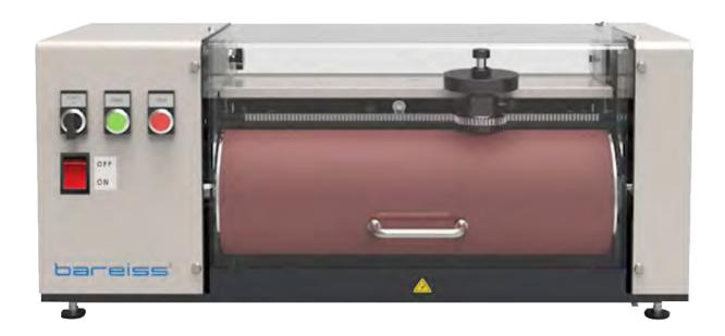
Rubber products such as tires, shoe soles, convevor belts are all prone to abrasive wear and therefore their physical ability to resist such wear determines their operational lifetime.
