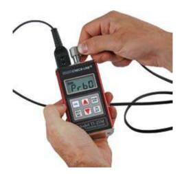
1. Connect probe and turn on gauge.
