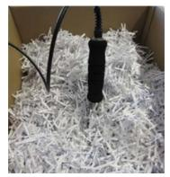
Plug the sensor into the material to measure and let it adjust for approx. 15 minutes. Switch on the humimeter RP6 and select the desired calibration curve. The display immediately shows the measuring result.
