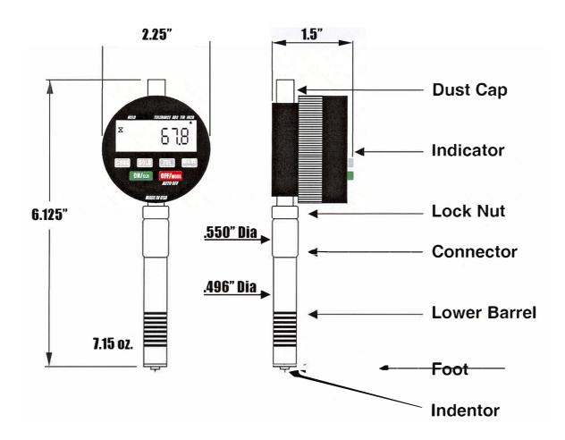
Note: There is a direct correlation between indentor extension and the display on the durometer. The display reads from 0-100 and the indentor extension is approximately .050".
