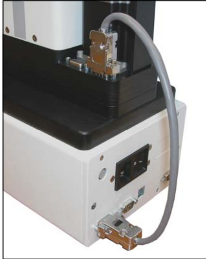
The illustration above depicts proper connection of the controller cable
