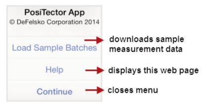
3 Select *Continue*. A list of available PosiTector probes (listed by connected probe type and serial number) will be displayed.
