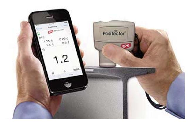
The PosiTector *SmartLink* measurement solution consists of a PosiTector App, PosiTector *SmartLink* device and compatible PosiTector probe.
