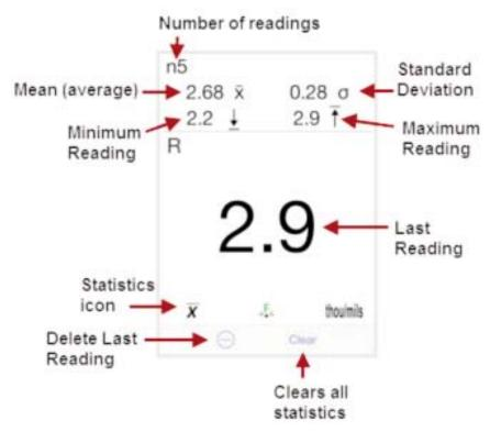
Deletes the last reading. Press *Clear* or the *LED button* on the PosiTector *SmartLink* to clear statistics.
