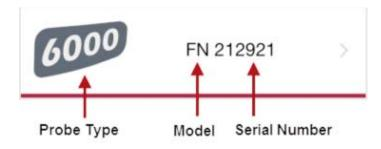
The probe model and serial number is engraved on the backside of the plastic probe connector (i.e. FN 212921).
