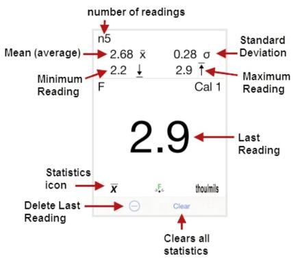
Deletes the last reading. Press *Clear* or the *LED button* on the PosiTector *SmartLink* to clear statistics.
