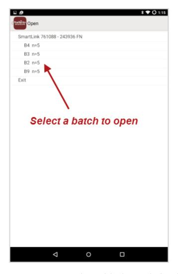
Additional measurements can be added to existing batches only if the original probe is attached to the PosiTector *SmartLink*.
