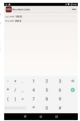
When HiLo Alarm is toggled ON, measurements will be compared to your defined HiLo limits.
