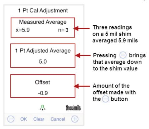
4 Select **OK** to accept the adjustment, **Clear** to start over or **Cancel** to exit without making any adjustments.
