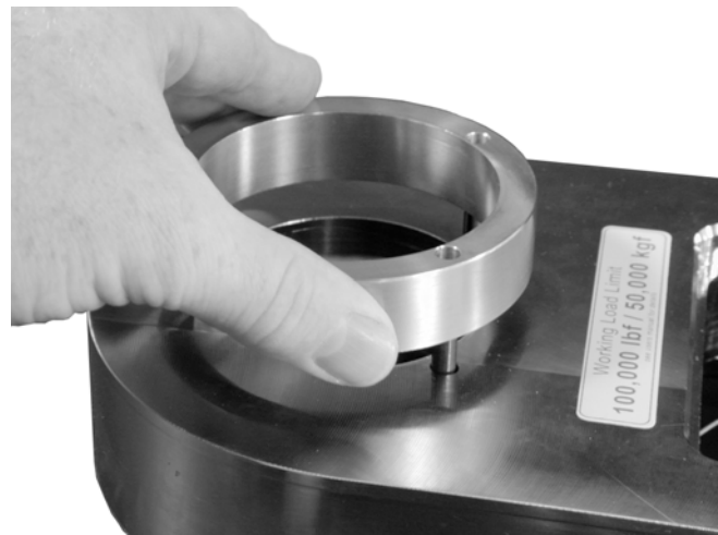
Figure 14 Placing second spacer on roll pins
