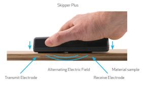
As there is a wide variation in the nominal electrical impedance of different material types, the instrument is provided with three selectable ranges which are optimized for testing (1) Hardwood, (2) GRP and (3) Surface Moisture.
