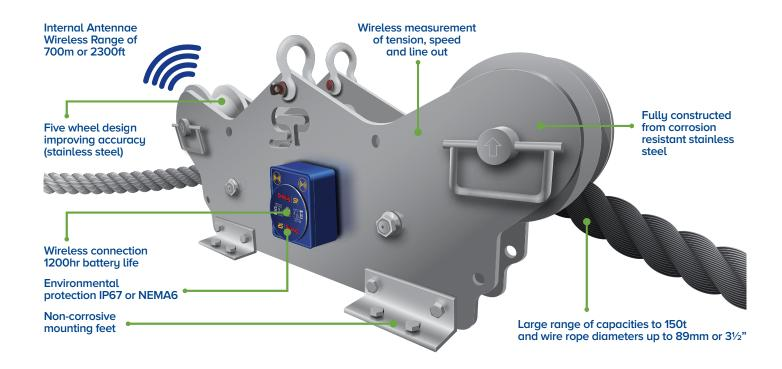
The TIMH range is a Wireless Running Line Tensiometer or RLTM built with dockside, marine, offshore, towage and salvage applications in mind. It is particularly useful when there is no anchor or dead end on the line to rig an SP Radiolink or Loadlink digital dynamometer. It measures tension force at speeds up to 20m/min or 65ft/min.
